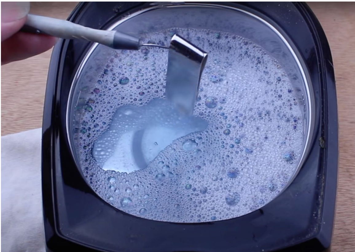
A Silver Money clip, being cleaned in the ultrasonic in between polishing stages. This is a vital stage before going on to final polishing.
