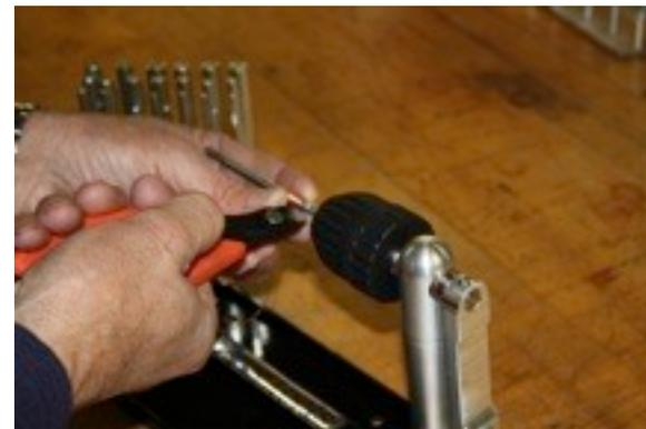
3) Remove the coiled wire from the mandrel. The end that is inserted into the arbor hole may be clipped or lifted out. Clip off or bend either end that may be sticking out above the coil. This will insure that the coil will lay flat in the V bed of the coil holder
