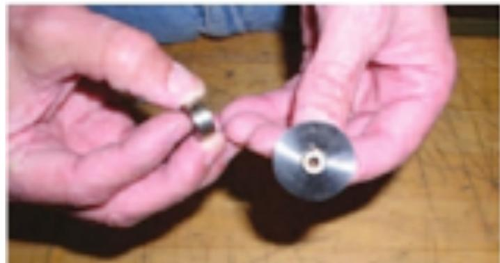
8) Slide the No. 30 Handpiece on to the handpiece Holder. Use the coil holder cover to center the blade, there is also an inscribed line that will aid you in centering the blade. Tighten the handpiece holding screws lightly, not excessively, located in the on top of the handpiece holder. The blade will now be centered on both the handpiece Holder and in the cutting groove on the Coil Holder.
