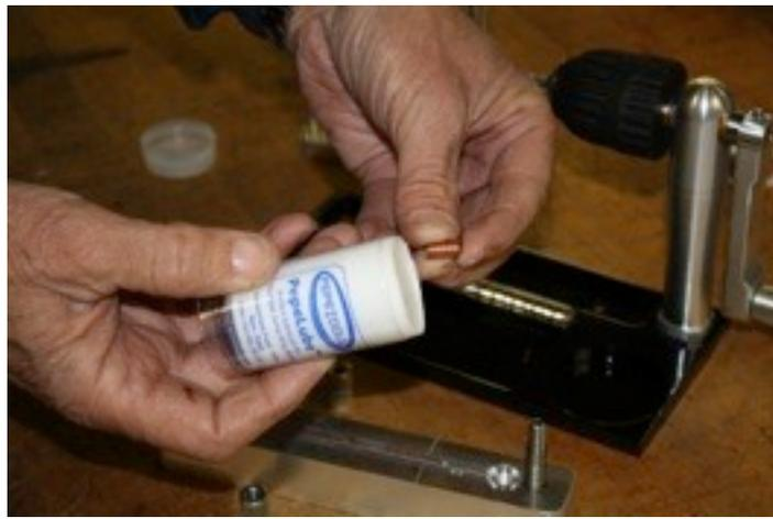
6) Place the coiled wire into the coil holding device making certain that the lubricated side of the coil is up and the coil butts up against the stopping bracket.
