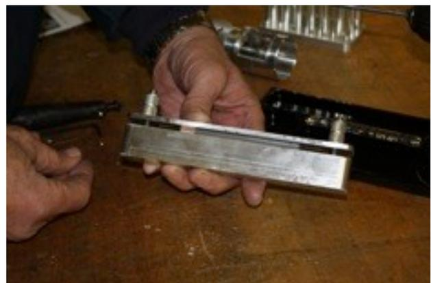
12) Place the coil holding device with the end that the coil is on against the stop. Place the hand piece holding collar with the HP and blade in place on the coil holding device. Run the flex shaft at full speed and with both hands and a light grip; pull the collar evenly towards you slowly. Once the cut is complete, remove the jump rings from the
