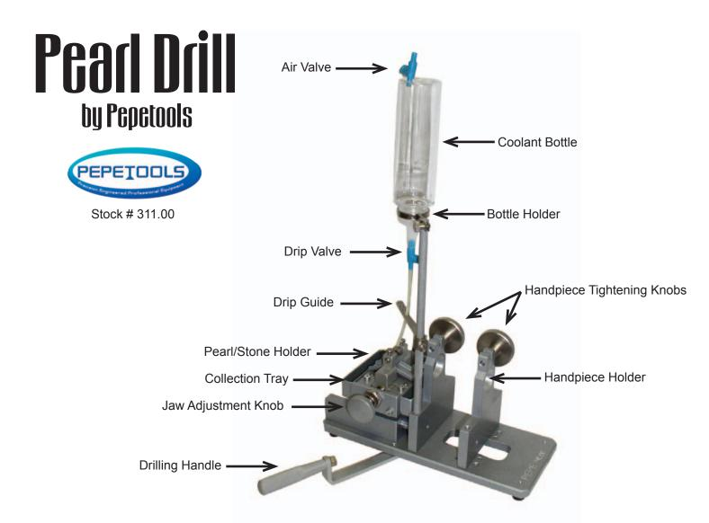
The new Pepetools Pearl Drill can be used to drill pearls or stone beads. It is made for use with a Foredom Flexshaft with a #30 handpiece. The unit includes The Pearl Drill, an optional drip cooling system and a set of 5 diamond core drills.
