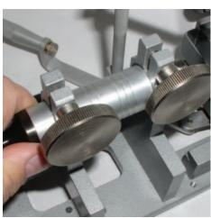
Turn the Handpiece Tightening knobs until the handpiece is firmly in place. Depending on bead size, you may need to adjust the placement of your handpiece to ensure that the bit travels far enough for sufficient drilling.
