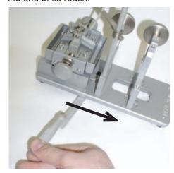
This will allow the table to spin freely. When the table is aligned with the drill bit it will snap into place on either side. So simply spin the table 180 degrees and push the handle back into drilling position.
