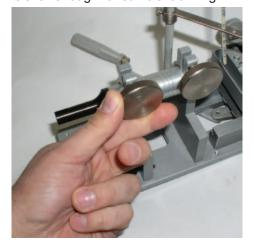
Place your bead between the jaws of the Pearl/Stone Holder and turn the Jaw Adjustment Knob until the bead is held firmly in place.
