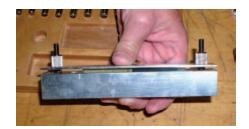
11) Secure a stop for the coil holding on a bench. This is necessary so that you may have both hands free when cutting the jump rings.
