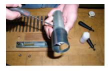
9) Place the cover over the coiled wire and replace the hold down nuts. Hold the cover down with your fingers right over the coiled wire. Tighten the nuts firmly but not excessively. Be certain that the cover is level over the coiled wire.
