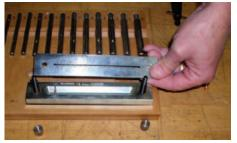
5) Rub Pepelube on one side of the coiled wire from end to end. This special lubricant is necessary as it lubricates the cutting blade and aids the cutting process.
