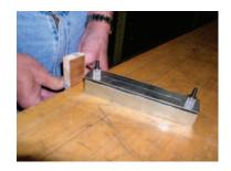
NOTE: The top of the coil holder fits completely down iin only one direction. This is only an issue when cutting small diameter jump rings, but be sure to double check that the top slides down flush with the base when placing the top on.
